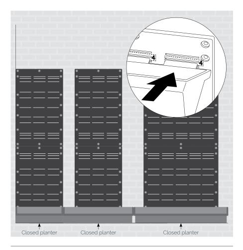
If the bottom row of **<u>closed</u>** planters is fully placed, start placing the other planters from bottom to top and then from left to right.
