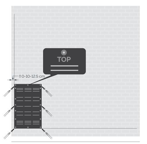
Determine the right distance between the grids before affixing the next grid. First place the bottom row.
