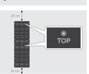
If you want to assemble a wall with non-standard dimensions, you can reduce the grids by cutting them to size along the sawing lines with a saw.
