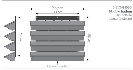
6NXGAM75D Module **bottom** The bottom planter is closed
